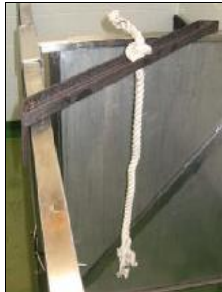
Fig 2. Corner bracket for suspending rope
