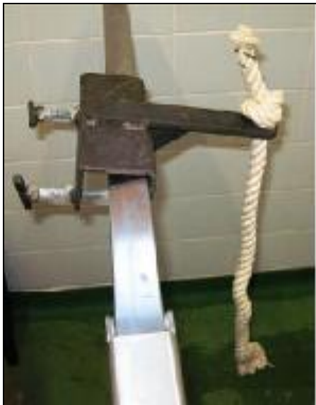
Fig 1. Adjustable wall bracket for suspending rope
